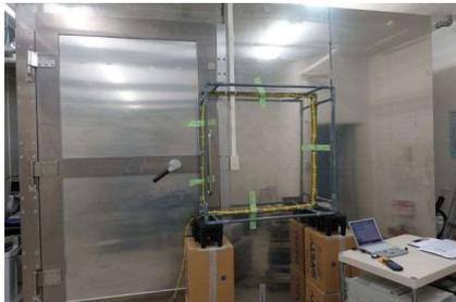
FIG. 1. Three-layered MSR developed in this study.
