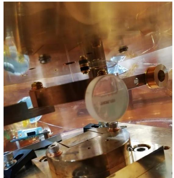
FIG 2. Picture of torsion pendulum, with attached mirror for optical lever readout, and coils for coil-coil actuation. The sapphire fibre used for suspension is 1 mm in diameter
